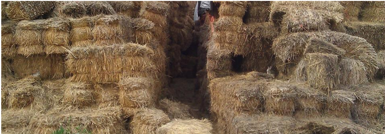
This photograph is of a 13-foot tall straw-bale pile after approximately one year of environmental exposure in Boulder, County, Colorado. Note the structural collapse, instability, straw dispersion and numerous rabbits that are visible. Several rats and one large bull snake were observed when the photo was taken at mid-day on 28 May, 2011.
